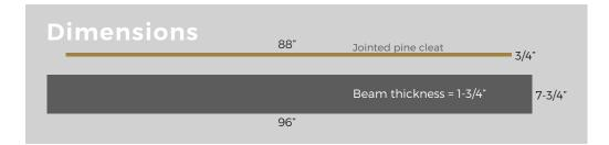
1. Install the supplied wood strip to your ceiling / wall using appropriate glue and hardware\*. Always pre-drill the wood strip to prevent cracking / splitting. Use a countersinking bit so the screw head does not protrude (Richelieu SKU# 31202004). Make sure the wood strip stays straight while installing.
