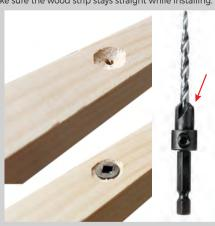
2. Insert the baffle over the wood strip and secure on both sides using glue with nails or screws\*. Always pre-drill if using screws.
